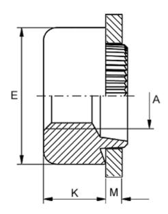
Female thread A = M14Height K = 10.0Outer diameter E = 25.0Plate thickness = 0.5 to 0.6
